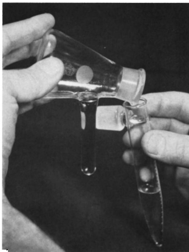
FIG. 1. Modified flask for cleavage of lipids and separation of products, in position for separation of immiscible phases.
